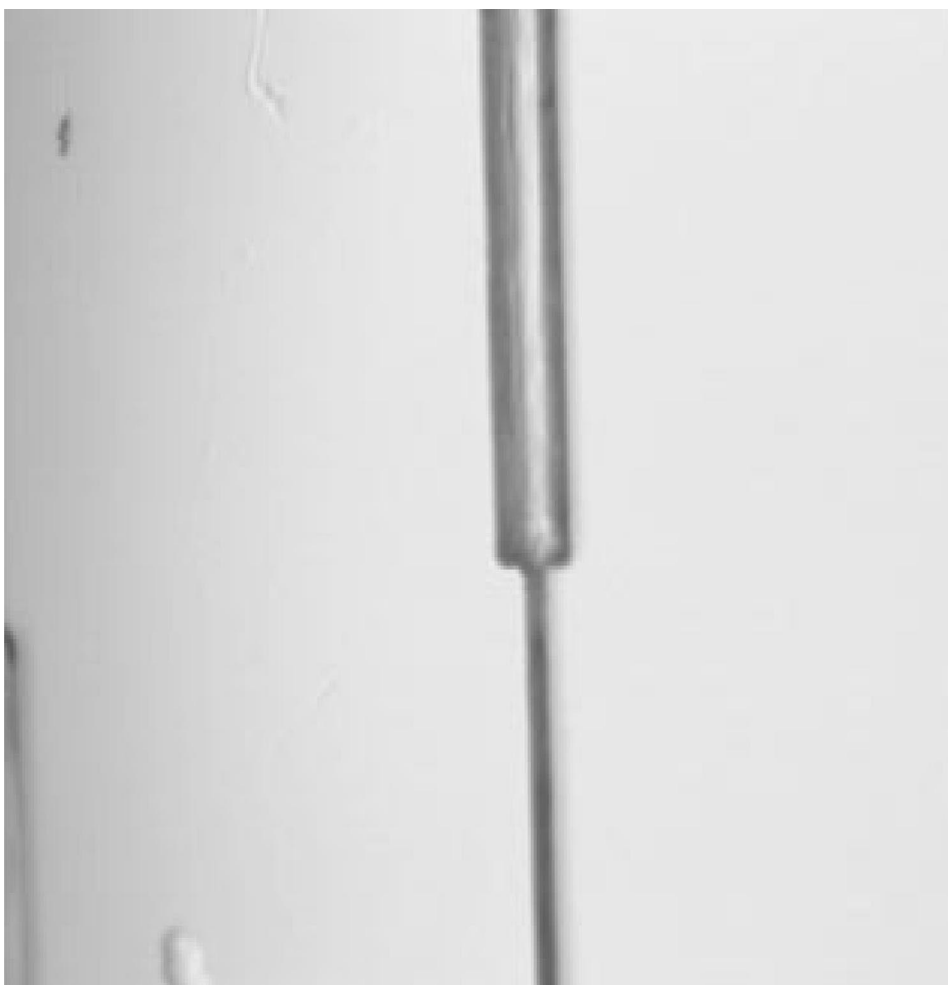
Fig. 5. Optical micrograph of a fused-silica capillary inserted into a micro-channel fabricated in PMMA. The capillary possessed an O.D. of 55 \mu\text{m} and an I.D. of 20 \mu\text{m} .
